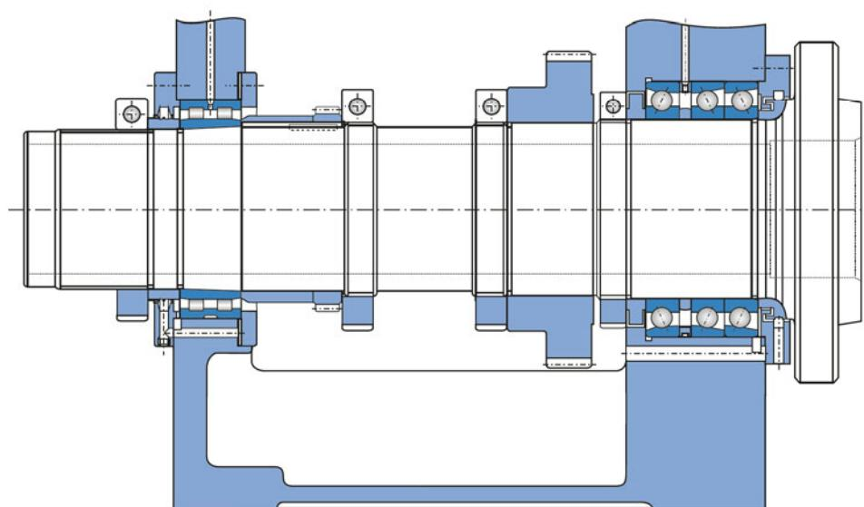
Fig. 27 High rigidity lathe spindle
