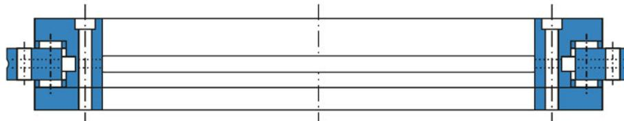
Fig. 10 Axial/radial bearings YRT
