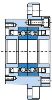
Fig. 9 Ball screw support bearing units
