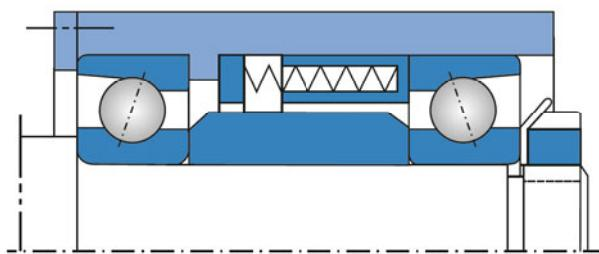
Fig. 14 Constant pressure preload
