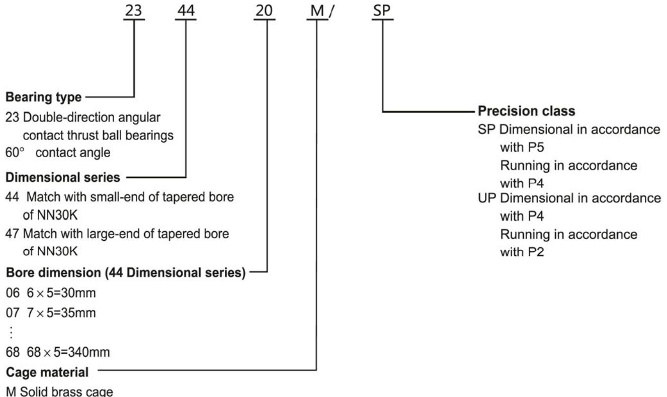
Double-direction angular contact thrust ball bearings
