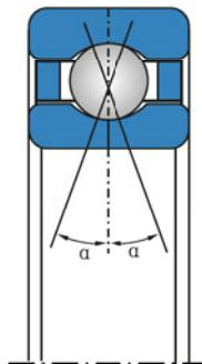
Fig. 11 Four-point contact ball bearings for turbo charger
