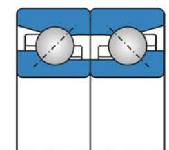
Fig. 4 High-speed angular contact thrust ball bearing structure
