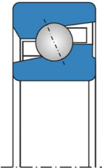
Fig. 7 Ball screw support bearings
