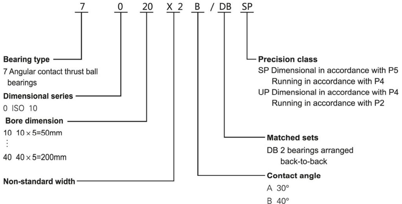
High-speed angular contact thrust ball bearings
