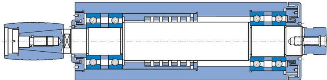
Fig. 29 Spindle for bore diameter grinding machine
