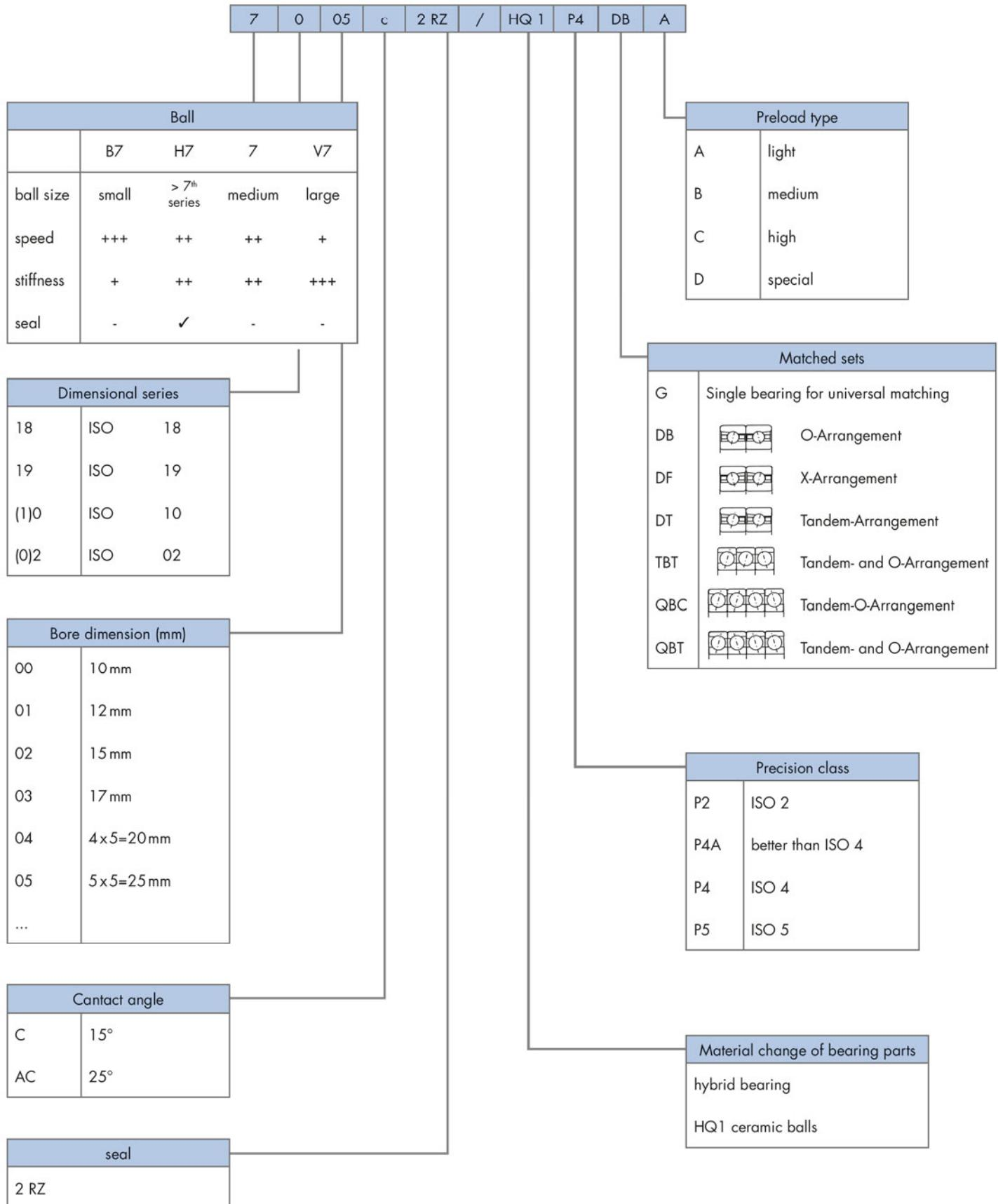
High-speed angular contact ball bearings
