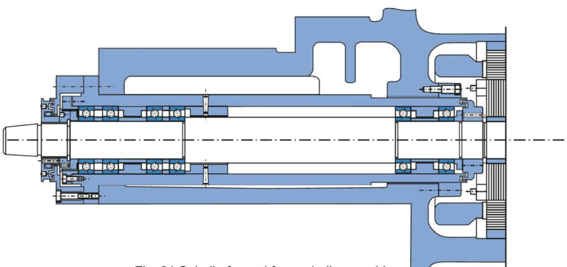
Fig. 31 Spindle for end face grinding machine
