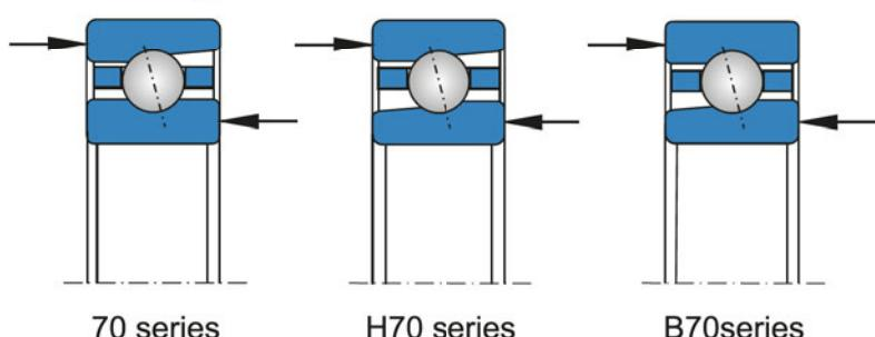
Fig. 20 Load-carrying directions of angular contact ball bearings
