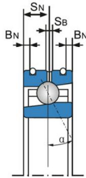
Angular contact ball bearings with direct lubrication
