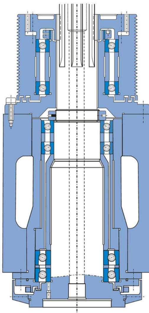
Fig. 25 Vertical lathe spindle
