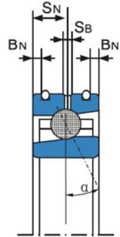
Angular contact ball bearings with direct lubrication (ceramic balls)
