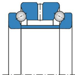
Fig. 3 ZYS Double-direction angular contact thrust ball bearings
