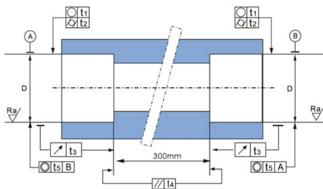
Fig. 15 Fitting shaft and fitting housing
