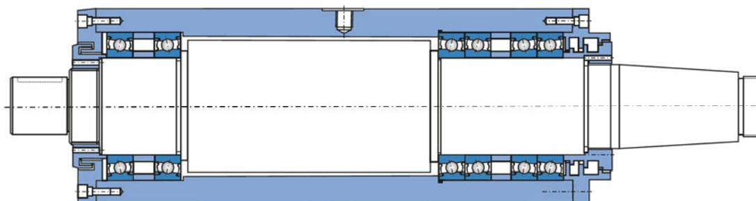
Fig. 30 Spindle for outer diameter grinding machine
